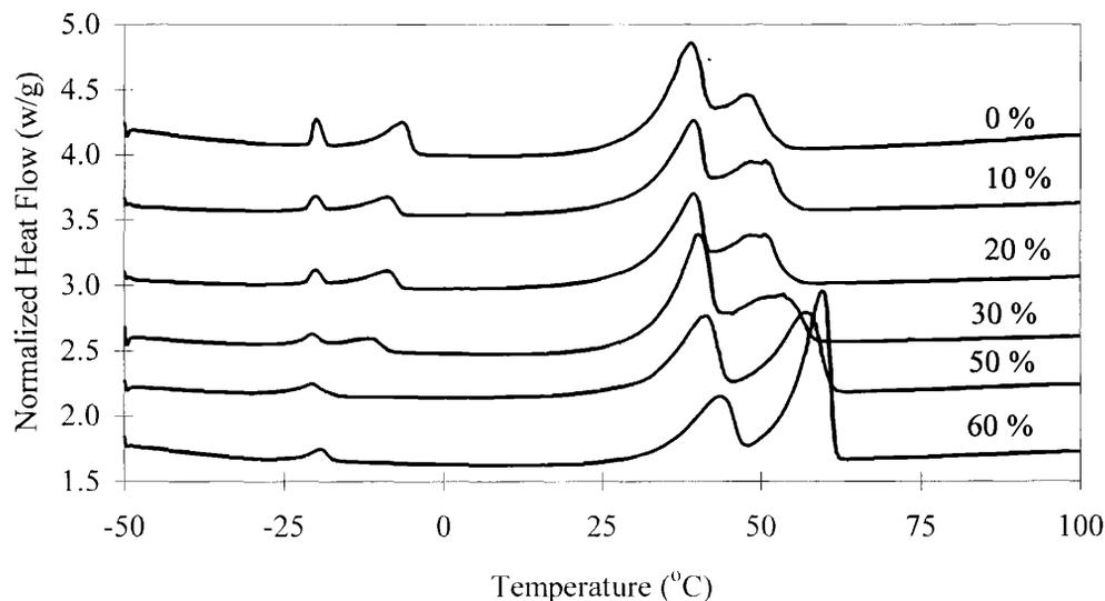
Figure 7. Representative thermogram showing the effect of percentage of triglycerides in the model sebum. Numbers on the side of thermograms indicate the percent of triglycerides.
