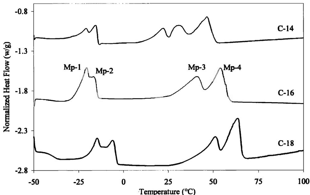
Figure 3. Thermogram showing the effect of carbon chain length in the model sebum (ratio of unsaturation to saturation 1:1).
