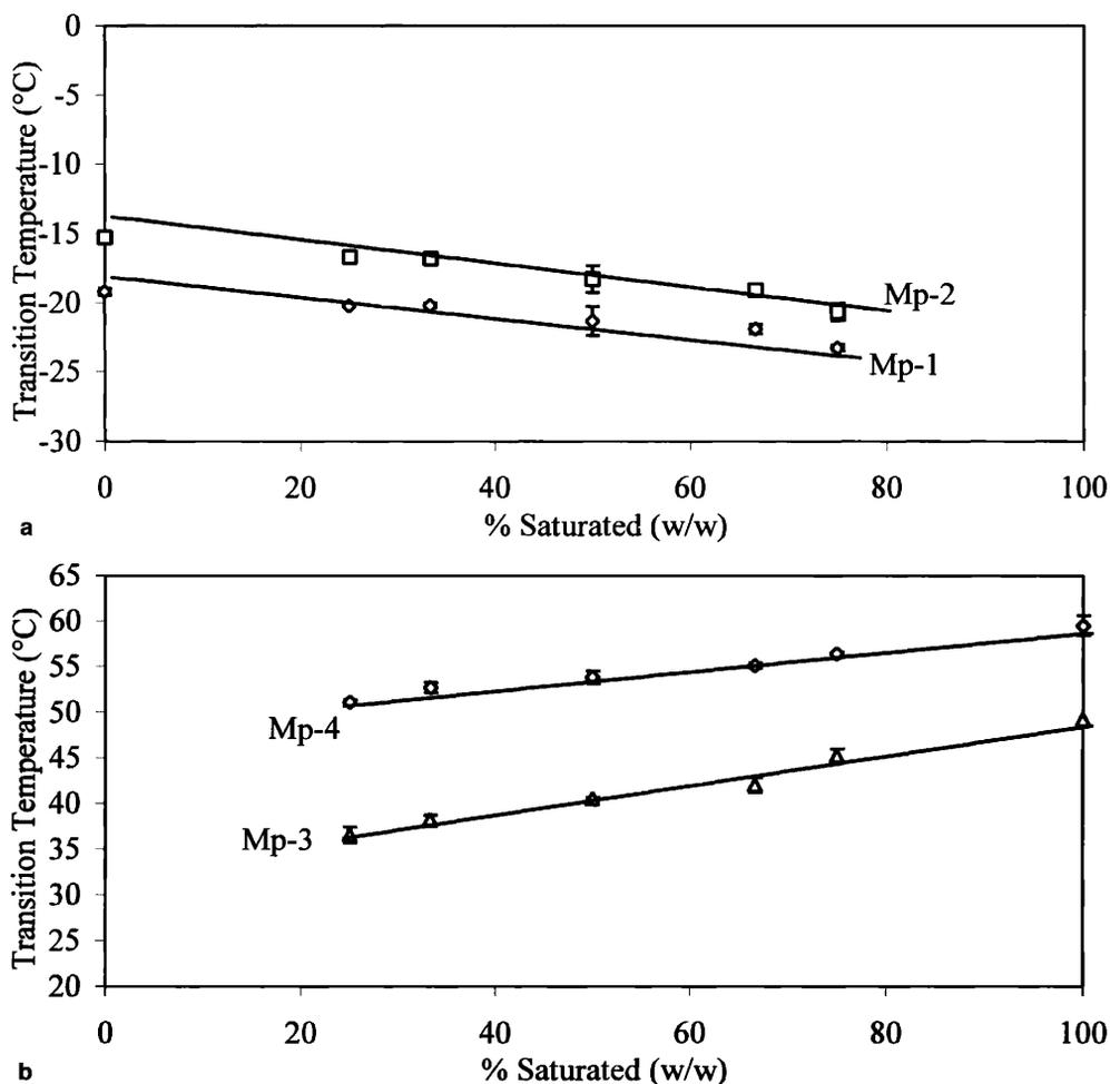
Figure 6. Effect of percent saturated on transition temperatures (a) Mp-1 and Mp-2 and (b) Mp-3 and Mp-4 for C-16. Error bars indicate the standard error of the mean of three replicates.
