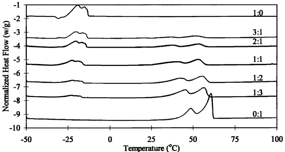
Figure 5. Thermogram showing the effect of percent saturated in the model sebum for carbon chain length 16. Numbers on the side of thermograms indicate the ratio of unsaturation to saturation.
