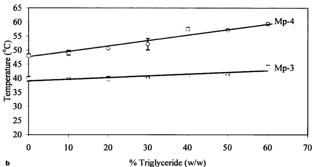
**Figure 8.** Effect of percentage of triglycerides on the transition temperatures (a) Mp-1 and Mp-2 and (b) Mp-3 and Mp-4 for C-16 (ratio of unsaturation to saturation = 1:2). Error bars indicate the standard error of the mean of three replicates.
