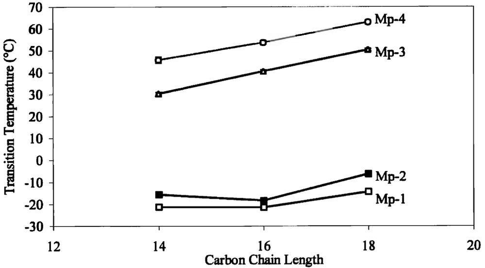
Figure 4. Effect of carbon chain length on the transition temperature (ratio of unsaturation to saturation 1:1). Error bars indicate the standard error of the mean of three replicates.
