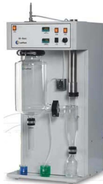
Fig. 4. Laboratory Scale Spray Dryer (Keison International plc, 2005)
